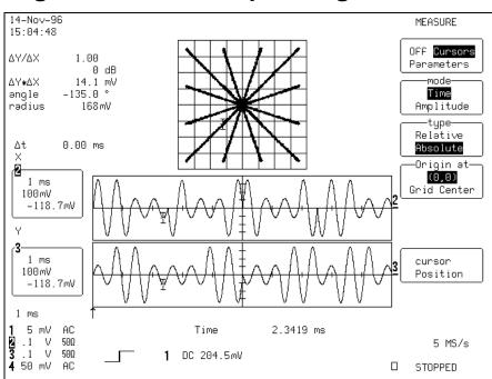
Figure 1 - Trace 2 shows the in-phase (I) component and trace 3 the quadrature (Q) component of a 16 QAM signal. The state transitions are shown in the X-Y diagram. Note that cursors mark a typical peak in the I and Q signals and simultaneously measure the phase and amplitude (radius) of the resultant vector sum.
